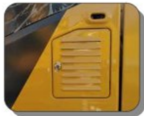
AC Filter Location
